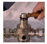
All Malgorani pressure reducers are tested before being packaged; during the proof they are pre-set at the outlet pressure of 3 bars; outlet pressure can be easely adjusted once the pressure reducing valve in installed on site.
